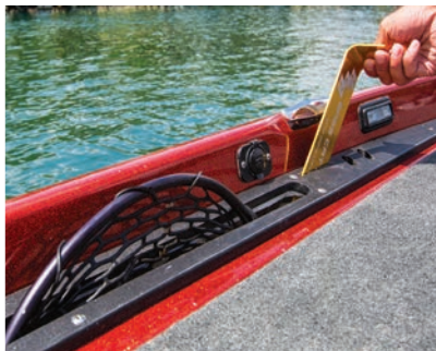
Integrated net, ruler, and tool holder on deck
