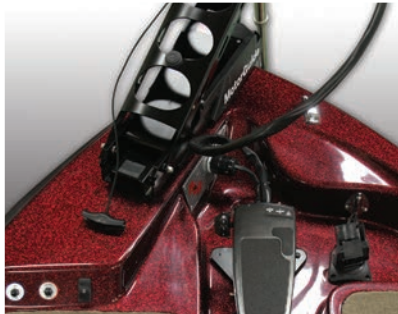
Recessed, low fatigue trolling motor well
