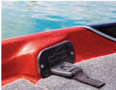
Standard retractable boat buckle straps on deck
