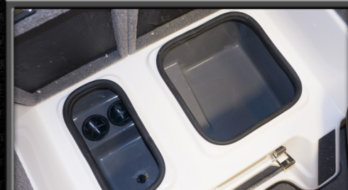
The front deck step is home to a day box, and large cooler with a raised sandwich tray.
