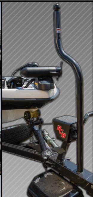
Our double wall, laser cut pivot tongue system is absolutely the strongest pivot assembly in the industry. A dual pin safety hinge will outlast all others on the road today.
