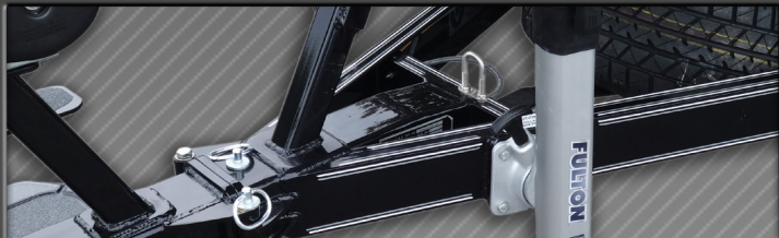
Our double wall, laser cut pivot tongue system is absolutely the strongest pivot assembly in the industry. A dual pin safety hinge will outlast all others on the road today.
