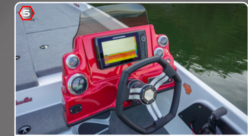
Rigid dash assembly capable of flush mounting 12" displays. Custom switch panel and 6X steering wheel.
