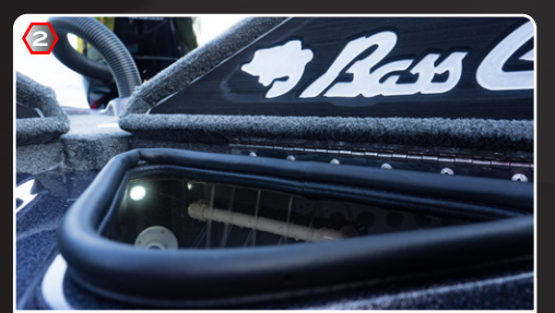
2 Lighted triangular livewells with advanced filtered spray bar aeration system for minimum slosh and high survival rate.
