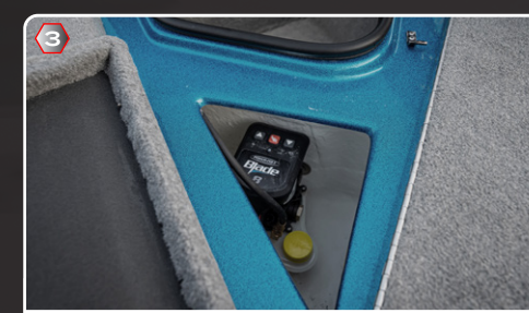
3 Dedicated anchor pump compartments with storage tray inserts.
