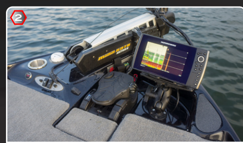
2 Adjustable foot pedal placement to fine-tune your stance on the front deck.
