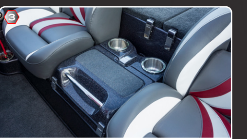
3 All-fiberglass center console/step box that flips up to expose a second insulated cooler underneath.
