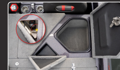
4 Rear deck storage re-shaped to accommodate dedicated anchor pump on both sides.
