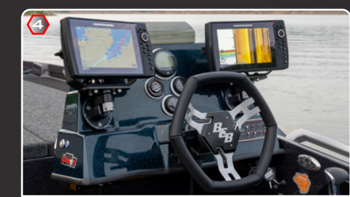
4 Updated all-fiberglass dash with new dual graph mounting layout.
