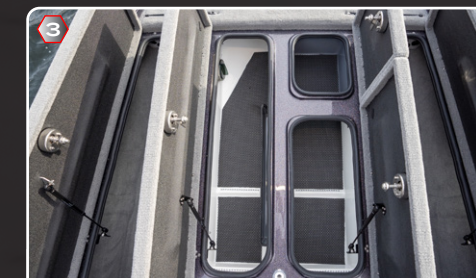
3 Unique coffin-style lid configuration to optimize accessibility and storage options.
