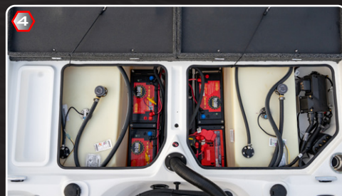
Balanced rear compartment with twin 30gal fuel tanks and fold flat, removable access panels.
