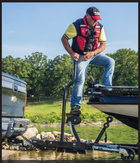
S-Bend grab post and custom offset fiberglass tongue step for easy access to the front deck.
